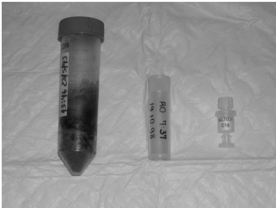
Fig. 1. Sizes of storage containers for storing and shipping muriqui fecal material to the United States. The container on the left is a 50-ml conical polypropylene tube for collecting fecal pellets and covering them in alcohol. The middle tube is a polypropylene container for storing fecal steroid extracts (5 ml of 50:50 ethanol : water). The column on the right is an SPE tube for storing steroids only, since the fecal material has been eliminated. This SPE tube has a top and bottom cap to keep the steroids moist.
